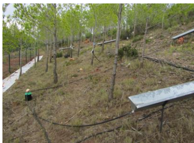
Gutters and tipping-bucket
