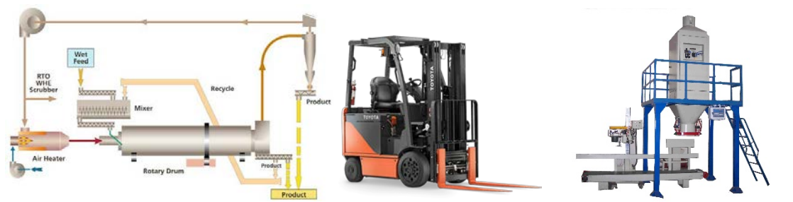
Figure 1: Conceptual scheme of a pellet rotary dryer (left), a fork-lift 4x4 (centre) and an automatic bagging system (right).
